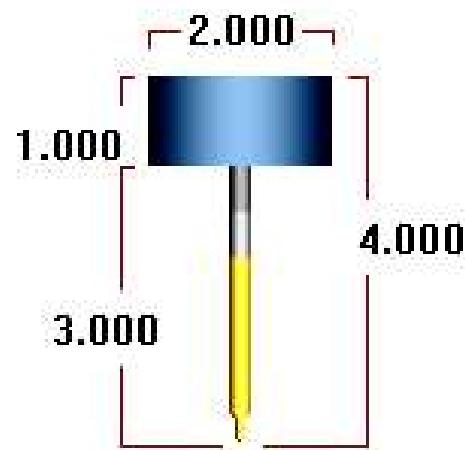
USED BY OPERATION: # 8 8 - C-Axis Cross Drill - Drill/Counterbore
